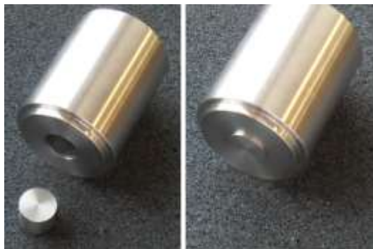
Figure 10: Putting the plug into the bottom of the mold
