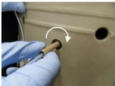
Figure 6: Connecting the loading connector to the check valve
