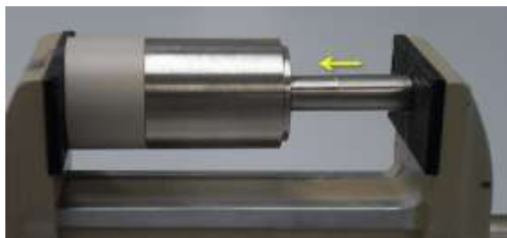
Figure 13: Removing the pellet from the mold by using the spacer of the pellet pressing tool
