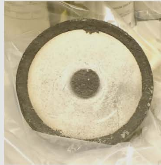
Base of broken graphite plug showing base of fused U ring
