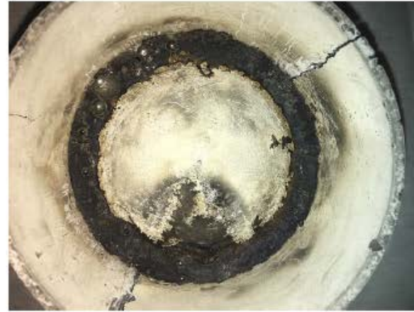
Casting surface showing oxidation and cavities
