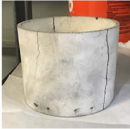
Graphite mold with ytttria wash post cast
