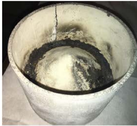
Casting surface showing oxidation and cavities
