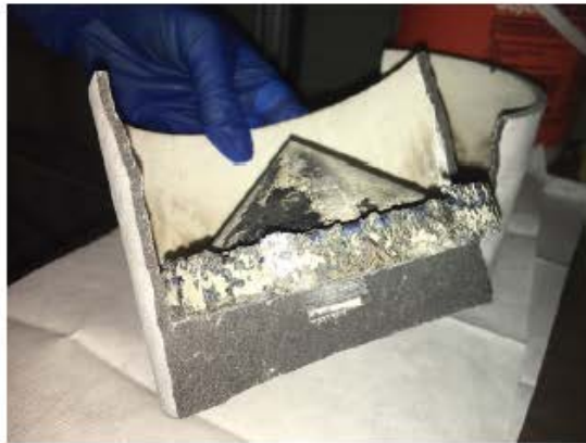
Graphite mold with ytttria wash post cast
