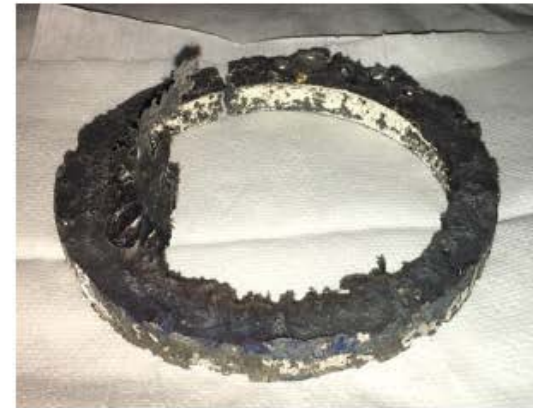
Casting surface showing oxidation and cavities
