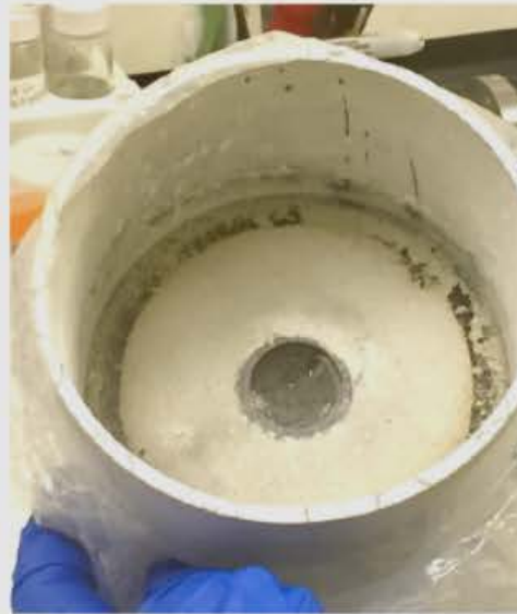
Base of broken graphite plug showing base of fused U ring
