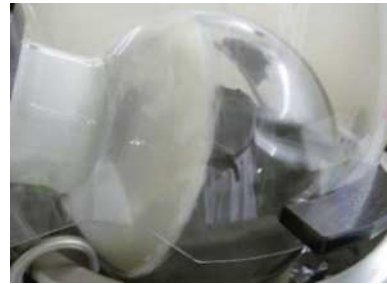
Beginning of the reaction between sulphur and metallic mercury
