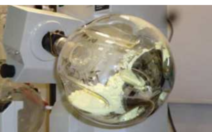
Stabilization process of metallic mercury by sulphur
