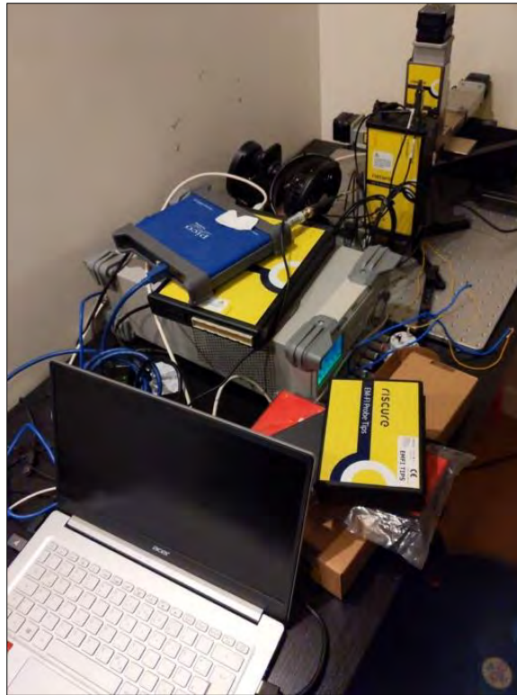
Figure 12: Setup used for FI during the second approach
